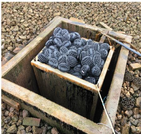
Figure 2: Concrete test bed containing SuperBiomedia™ in trickling filter placed inside existing trickling filter.
